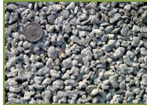
**Porous Asphalt** -- Porous asphalt is typically standard hot-mix asphalt that contains less sand than traditional asphalt. Like porous concrete, it also contains air pockets that allow water to seep through it. Porous asphalt is commonly lighter in color than conventional asphalt and cooler during hot weather.
