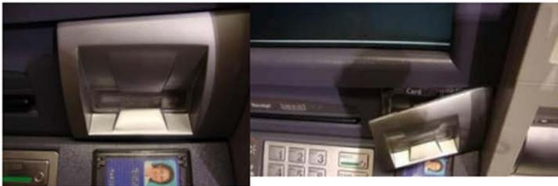
Skimmer placed over card slot & Partially removed
